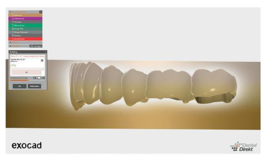
The exocad® "production blank" module or nesting with DD smartCAM 2.0 makes it possible to individually adjust the degree of translucency in the incisal area of the restoration
